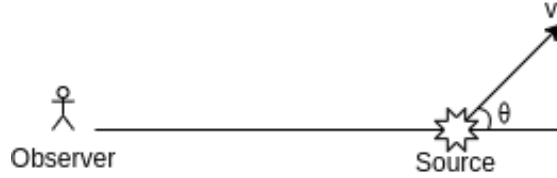
Figure 4: Doppler shift for a moving source
